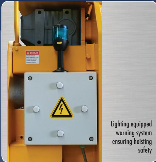
Lighting equipped warning system ensuring hoisting safety
